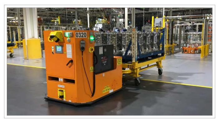
The Fori Tugger and Dock N' Lock AGVs are high capacity vehicles that are designed to replace fork lifts or standard man aboard Tuggers for material handling. The Tugger AGV is capable of weights up to 35,000 lbs. and have been designed to accommodate existing cart and hitch designs. The Tugger AGV is also upgradeable to a Dock N' Lock AGV which offers increased automation versus the standard Tugger AGV.
