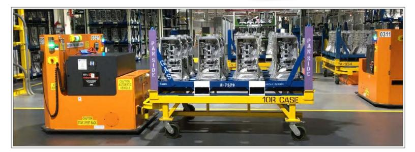
The vehicles overall towing capacity is 35,000 lbs. The total capacity can be customized by utilizing different options of off the shelf drive wheel, gearbox and motor combinations. A Siemens Safety PLC is used for safety and vehicle control, resulting in an open controls architecture.
